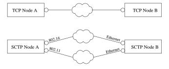
Figure 1: An SCTP Association vs. a TCP Connection
